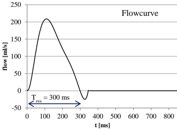
**Fig. 3** Systolic flow cycle profile for one cycle of duration  $T = 850$  ms, see e.g. Brücker et al. [2]. 35 ml per beat were pumped during opening and closing of the heart valve within a cycle of  $T_{sys} = 300$  ms.
