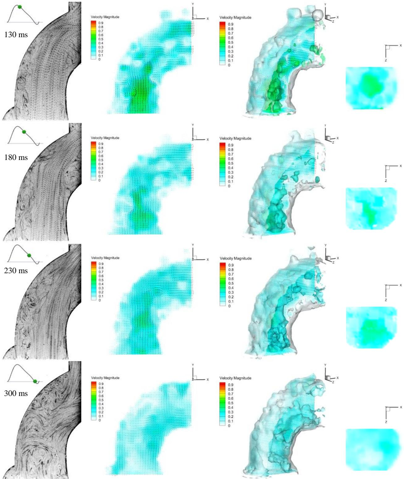
**Fig. 5:** Visualizations of the particle movement and the velocity fields at six different phases of the systole cycle. First column shows multi exposure picture of particle displacement for one light-sheet (LS) from earlier measurements [see 6]. The LS is aligned in the middle of the aortic arch. Column two to four showing the analyzed velocity field, the XY-plane, an isometric-view with different iso-surfaces and the XZ-plane.
