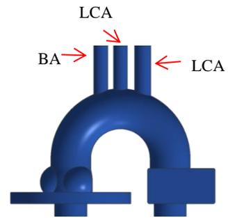
**Fig. 1** CAD - Model of the aortic model including the cerebral vessels.
