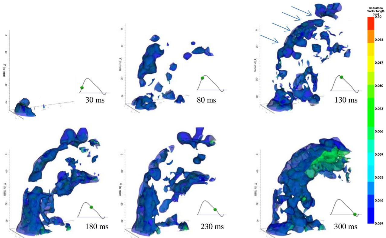
**Fig. 6:** Visualization of iso-surfaces for six different time steps referring to Fig. 5. Three iso-surface regions are shown, with velocities of 0.01 m/s (blue), 0.05 m/s (green) and 0.1 m/s (red). Shortly after the opening of the valve, the velocities in the whole arch range over 0.1 m/s, except in the right bulb. With growing time, low velocity regions are developing on the walls and in the inner regions of the aorta.
