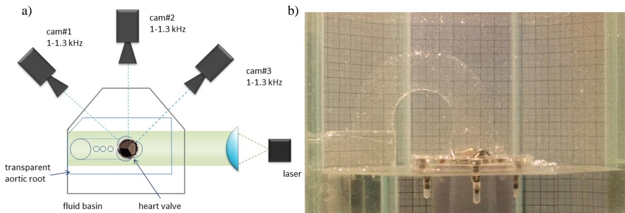
**Fig. 2a)** Schematic top view of the experimental set-up: the laser illuminated the volume inside the aortic arch, while three high speed cameras recorded the individual particle movement at 1 or 1.3 kHz. The glass tank was filled with a water-glycerin solution to ensure a refractive index matching between the transparent aortic model and the fluid. **b)** Refractive index matching of the transparent silicon model (Elastosil RT 601™).
