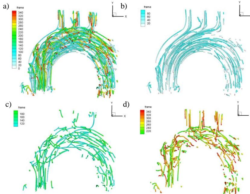
**Fig. 4:** View on the particle tracks. a) Complete heart valve cycle. b) 1<sup>st</sup> period (0-100 frames). c) 2<sup>nd</sup> period (100 – 200 frames). d) 3<sup>rd</sup> period (200 – 347 frames). The colorbar presents the different frames.
